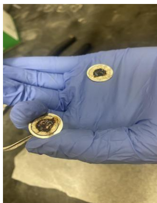
Figure 5 DOBHTP-PEGMEMA, after CV test at 60°C, opened coin cell
