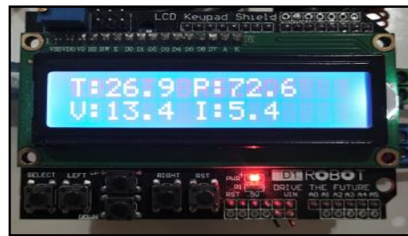
Figure 3 Arduino-based real-time data acquisition unit.
